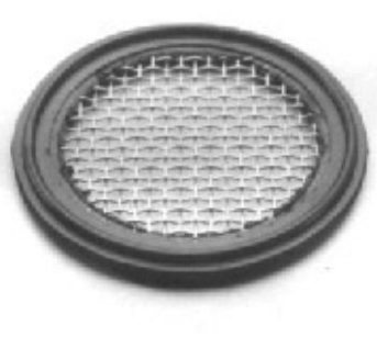
SCREEN GASKETS 40MP-US Type 304 Stainless Steel, .025 Dia. Wire Width of opening .078 in. between wires—(104 STAPs) 100 openings per sq. in. Sizes Available: 1", 1½", 2", 2½", 3", 4", & 6"
