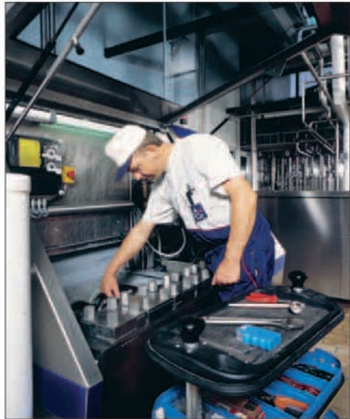
Easy-to-open doors and removable covers make maintenance easy and accessible in Tetra Alex 400 homogenizers.
