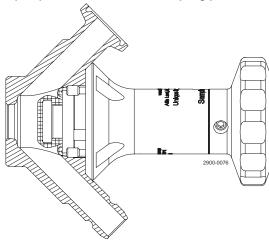
Manual valve: rotate the handle in a counterclockwise direction to open the valve. Pneumatic valve: open the valve by activating the actuator. This retracts the valve stem and membrane seal, which enables the product to flow freely through the open valve.
