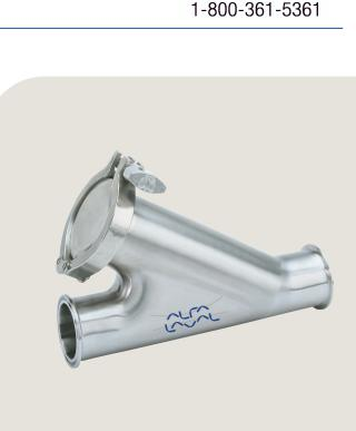
equalizes. The ball then returns from the "Y" branch of the valve and rests itself against the smaller diameter of the valve near its inlet. Should a reverse-flow situation occur, the opposing pressure of the fluid will seat the ball firmly against the inlet of the valve, preventing reverse flow.
