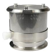
When filling or emptying a tank this valve relieves pressure or vacuum and seals under equal pressure. In addition, it includes an external stainless screen that protects against larger particulates from entering the tank. It includes a 1/4" FNPT port that allows inert gas to be pumped into the tank.
