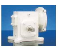
**Outstanding Features:** Precision ground worms of high quality alloy steel; accurate hobbed cast bronze gears; tapered roller bearings on output shaft permit maximum overhung load capacity; large oil reservoir for splash lubrication affords cool operation and oil seal design provides trouble free operation
