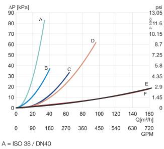
B = ISO 51 / DN50 C = ISO 63.5 / DN65 D = ISO 76.1 / DN80 E = ISO 101.6 / DN100
