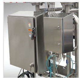
Electrical and Pneumatic Components Separated
